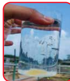
Floc formation and settling in reaction chamber
