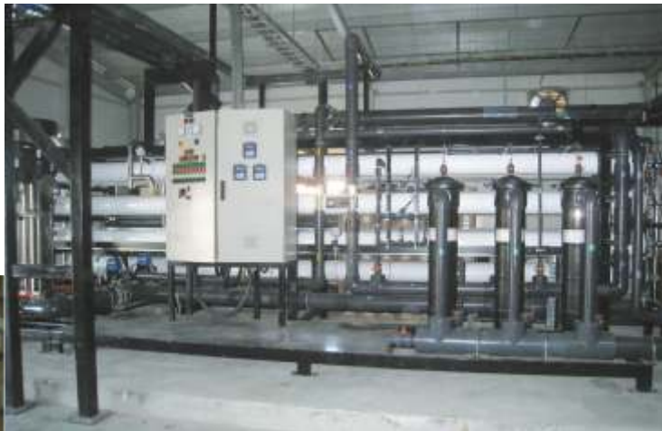
2 x 300,000 USGPD (2 x 1135 m 3 /d) brackish water treatment reverse osmosis plant supplied to Umm Al Quwain, Government of UAE
