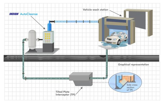
INDION AutoCleanse is a state-of-the-art system to treat and recycle vehicle wash effluent. The system enables you to save 80% water cost by conserving large volumes of freshwater. The system also meets stringent environmental discharge regulations.
