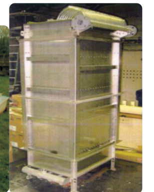
INDION Membrane Bio-Reactor
