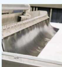
Belt Press for Iron Ore Slurry
