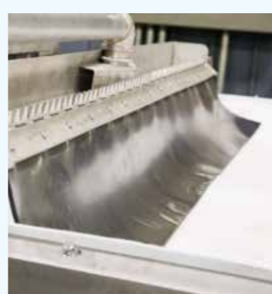
Belt Press for Iron Ore Slurry
