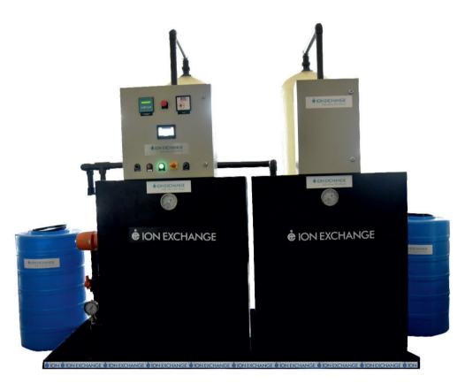
Indion New Generation (NG) Elegant is designed to produce high purity water required for boilers, pharmaceutical and electronic processes. Indion NG Elegant is skid mounted comprising of individual cation and anion unit. It incorporates counter current flow of ion exchange technology.
