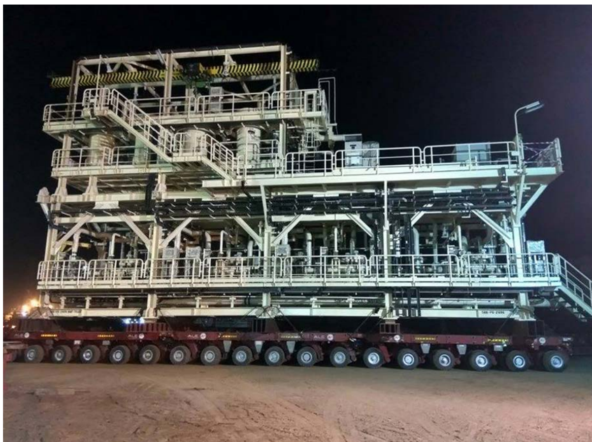
Complete assembled skid being moved on Self Propelled Modular Transporter (SPMT) from Fabrication Yard to Barge
