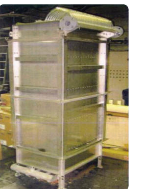
INDION Membrane Bio-Reactor
